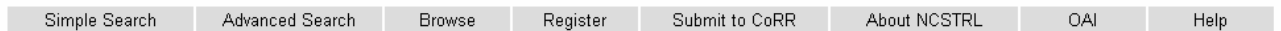
Figure 5. False cognitive affordances in a menu bar with links that look like buttons
