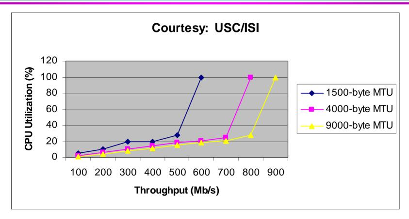
Note: The congestion-control mechanism does *not* get activated in these tests.
